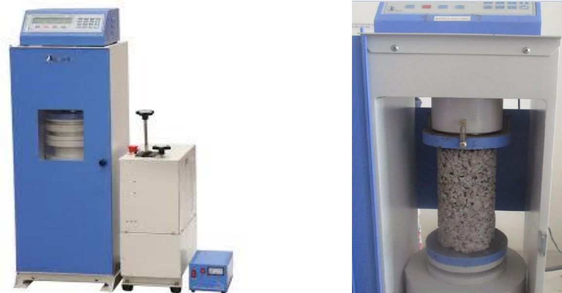
Figure 3. Compression testing machine, with 2000 kN loading capacity
