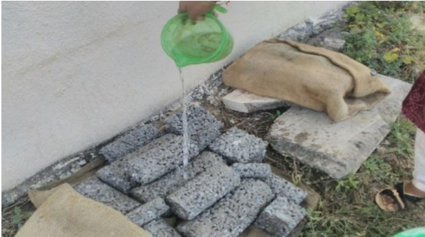
Figure 2. Samples wrapped in gunny bag for curing
