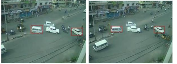
Figure.6. Moving Blobs Identified between Frame 1 and Frame 2 by applying Equation (1)
